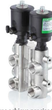
These direct-acting valves achieve precise temperature control in fermentation tanks. Each body is comprised of two valves with six ports to allow both the feed and return of media – allowing one component to control both hot and cold glycol flows.
