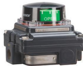
Breweries use a variety of pneumatically actuated ball and butterfly valves across their processes. Mounted on top of any pneumatic actuator, TopWorx switchboxes offer position indication and control for on/off valves. They have a variety of communication options such as ASi, Device Net, or Profibus, or can incorporate a proximity sensor such as the TopWorx GO Switch.
