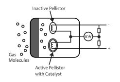
The SC310 provides versatile, robust, and field proven performance with the added feature of hydrogen gas detection. This catalytic bead sensor is self-compensating to environmental changes. Additionally, it is easy to install, calibrate, and operate.
