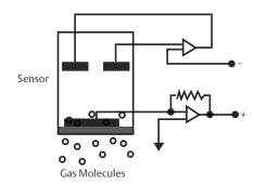
This dependable electrochemical sensor provides high specificity, fast response time, is easy to calibrate, and has a long life. This sensor produces more current as gas comes into contact with it.
