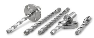
With its revolutionary design manufactured specifically to eliminate the concern of vortex induced vibration (VIV) that can lead to thermowell stem failure, the Twisted Square dampens vibrations by over 90%, drastically reducing the dynamic stresses experienced by the thermowell. This allows the Twisted Square to operate in process conditions that a conventional thermowell cannot.
