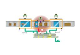
Zoned Safety capability enables isolation of up to three safety zones on a machine from one single valve system, improving productivity, and reducing cost and complexity.
