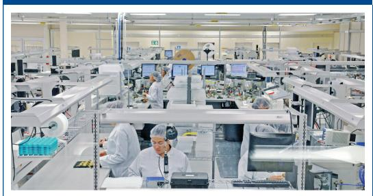
Our miniature solenoid valves are manufactured in ISO Class 8-equivalent clean rooms to eliminate contamination risks.
