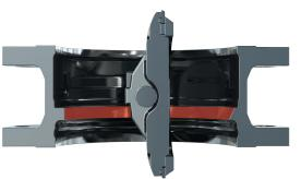
Full metal construction with solid seal rings in Nitronic 50 and wear-resistant Stellite Grade 21 seat overlays
