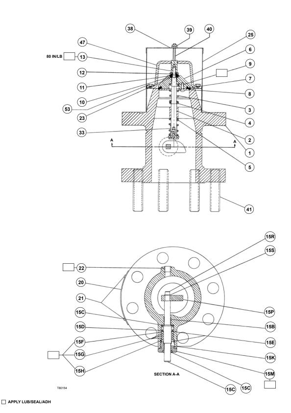
Figure 5. Type C403-24 Internal Valve
