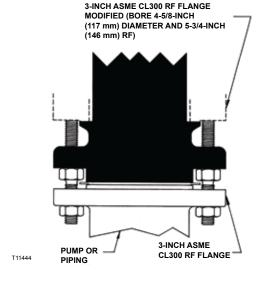
Figure 2. Tank Flange Dimensions
