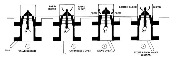
Figure 4. Operational Schematic For Types C403-24 (shown) and C404-24
