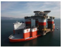
Dockwise Vanguard is designed for heavy marine transport and offshore dry docking. The length are 275 meter, draft submerged 31,5 meter and max water height above deck is 16 meter. Max lifting capacity 115.000 metric tons.
