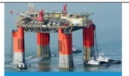
Four identical systems with operation possibilities locally in each column and centrally from the Ballast Control Room at the topside.
