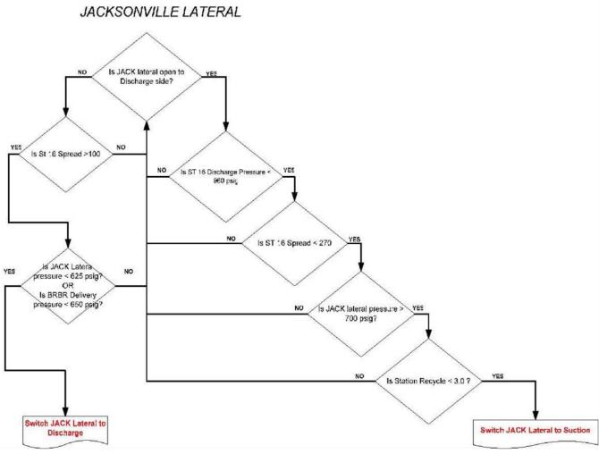
Figure 6. Jacksonville Suction/Discharge Switch Alarm
