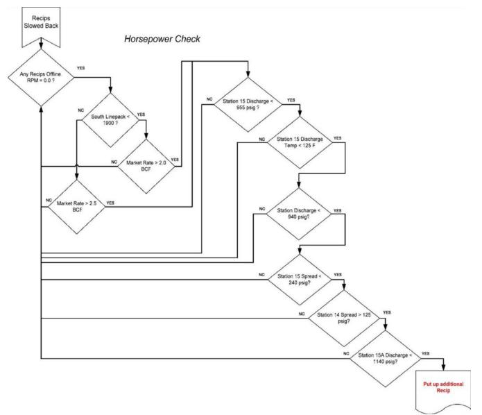
Figure 3. Additional Horsepower Required Alarm
