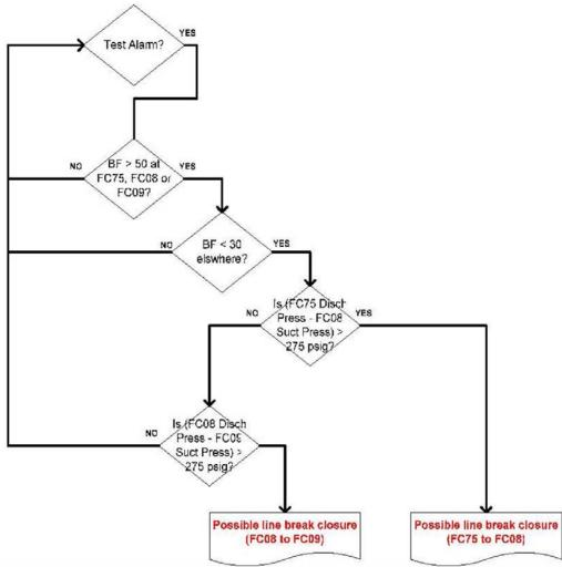
Figure 4. Line Break Operator Alarm
