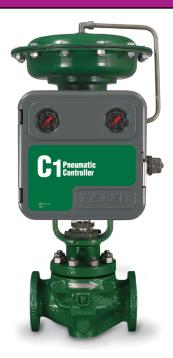
Each Fisher C1 pneumatic controller uses 1/10th of the natural gas of older, high-bleed models. A green label and green Bourdon tube symbolize the C1 controller's energy- and cost-saving benefits.
