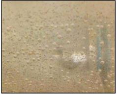
Sand covers the FDM tines, alarming the customer by generating an 'enhanced event' on a digital output
