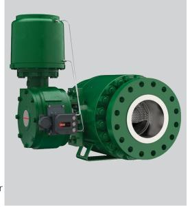
The solution involved retrofitting five hundred units to FIELDVUE digital valve controllers with low-bleed relay option. The relay enables low air consumption of 0.14 Nm³/hr. With its linkage-less, non-contact position feedback mechanism, there are no wearing parts so cycle life is maximized.
