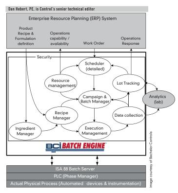
Middleware like the batch engine software shown in this diagram is often used as a transfer point for communications between plant control systems and ERP systems
