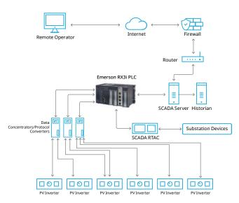
Flexible control solution is based on open architecture and supports multiple protocols.
