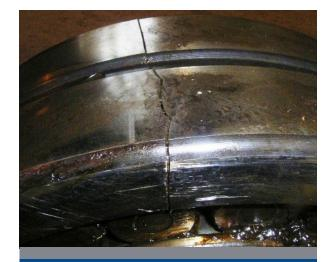
"When inspected, the outer race of the bearing was cracked and flaking. It was only a matter to time before this part failed during normal operation."
