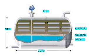
Figure 3: Drawing of installation in desalter tank showing emulsion layer and electrical grids.
