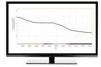
Each sensor provides continuous measurements of equipment thickness.
