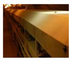
Image 3. Each of the nine conveyor belts had four bearing temperature measurements and four rub block temperature measurements that were handled by one Rosemount 848T FOUNDATION Fieldbus High Density Temperature Transmitter.
