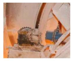
**Image 5.** Four Rosemount 648 (single point) Wireless Temperature Transmitters were placed inside the silos to measure bearing temperatures and motor currents.
