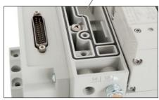
NOTE: Manifold Assemblies are factory set for internal pilot supply. To convert to external pilot supply install pilot supply seal screws 501 Series: 127-803.
