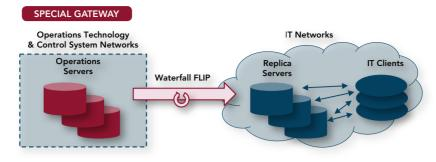
Figure 2. New unidirectional gateway allows temporary, controlled external inputs. Source: Waterfall Security Solutions.
