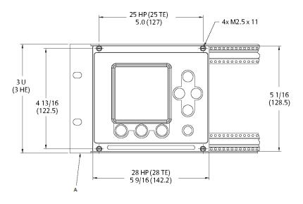
A. 19 in (483 mm) sub-rack conforms to EN 60297-3-101 and IEC 60297-3. Not included as part of the 3300/3500
