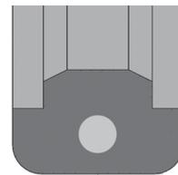
Perimeter resilient seated valves, like the PCS17 are bi-directional. With a perimeter seat, pressure against the gate is not required to create a seal, so testing is done in one direction only.
