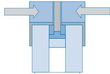
Polymer lined valves, like the M145, have bi-directional, pressure assisted seals. Because of this, they are tested in both directions with pressure pushing the gate against the seat.
