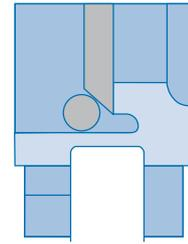
Metal-to-Metal seated valves, like the F220, are uni-directional and are tested with pressure pushing the gate against the seat.
