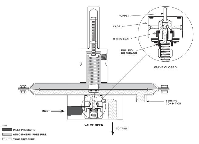
Figure 2. Operational Schematic
