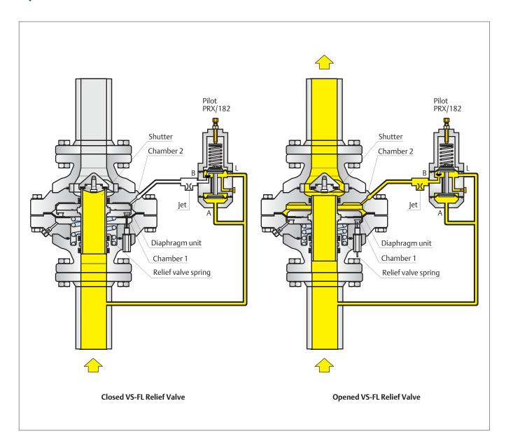
The diaphragm unit (permanently connected to the shutter) divides the relief valve actuator into two chambers.
