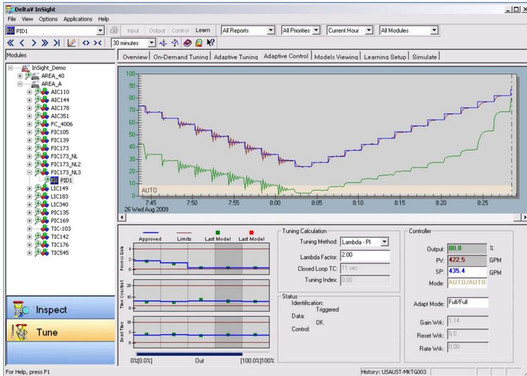
*DeltaV™ Adapt provides continuous adaptive control for any DeltaV PID control loop.*
