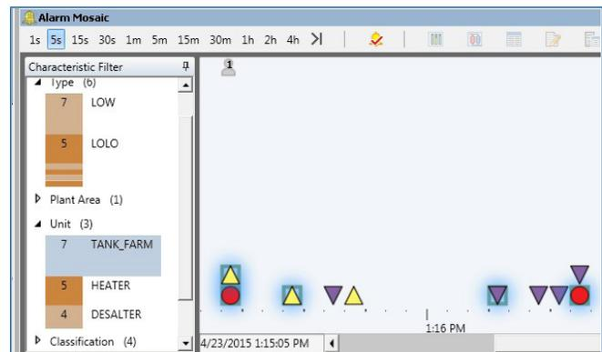
Alarm with common characteristics are automatically identified, enabling the operator to more easily comprehend the overall situation.
