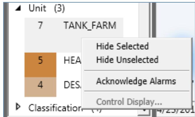
With a single mouse-click the operator can mass acknowledge, filter out, or select only the alarms with a shared characteristic.
