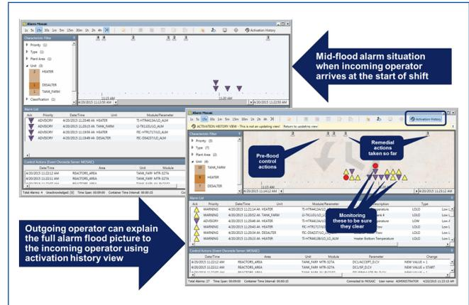
Shift transitions represent a critical moment, especially if an alarm flood is in progress. The Alarm Mosaic Activation History View allows the incoming operator to observe alarms and control actions from the prior shift.
