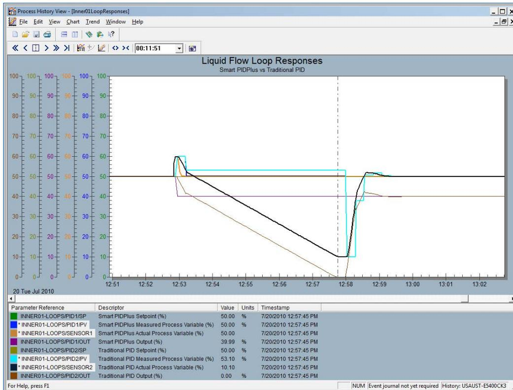
Figure 5 — Flow Failure Response of PIDPlus and Traditional PID (update time = 16 sec).
