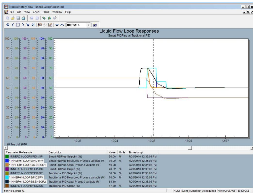
Figure 4 — Flow Load Response of PIDPlus and Traditional PID (update time = 16 sec).
