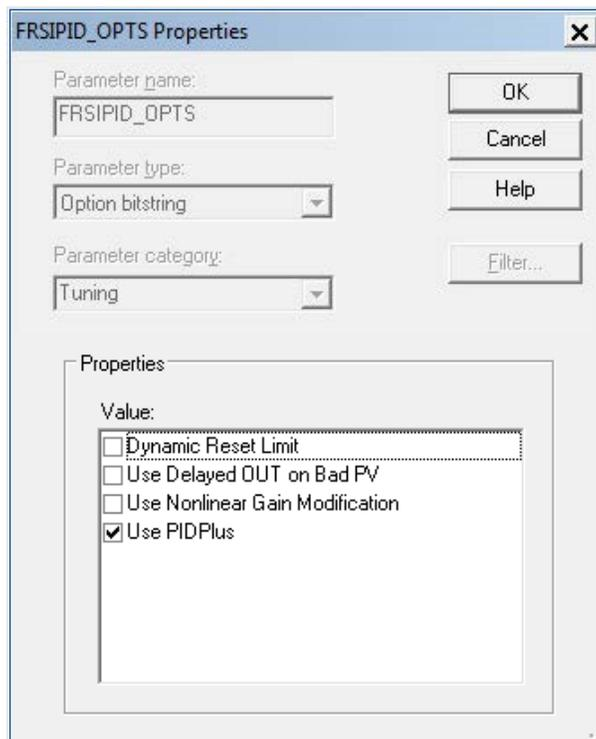
Figure 1 — PIDPlus enabled in FRSIPID\_OPTS for PID block.
