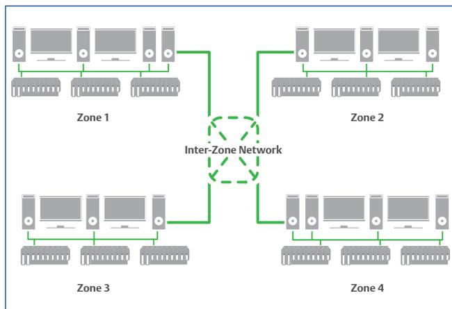
*The Inter-Zone Network is shown in bold green to demonstrate how multiple standalone systems can be connected via Inter-Zone Servers in each zone.*
