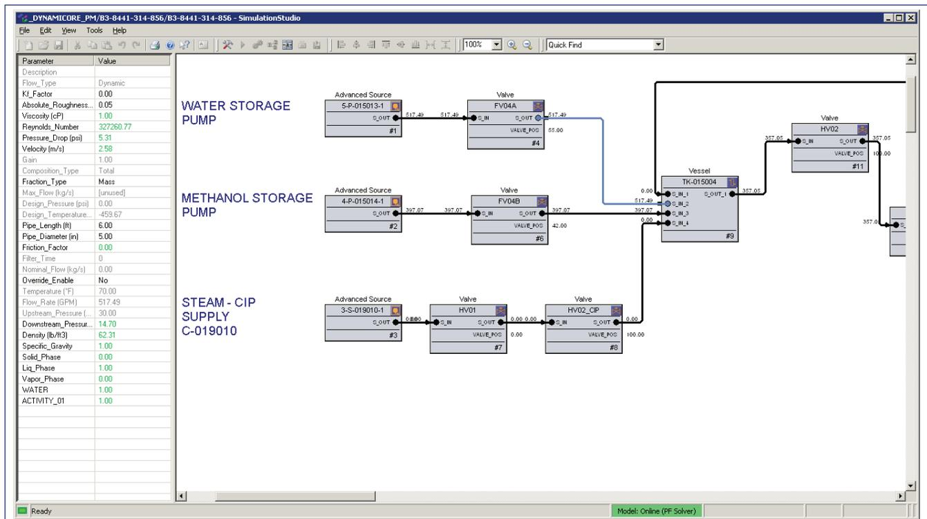
Unit operation objects are used to quickly develop accurate models for testing and training.
