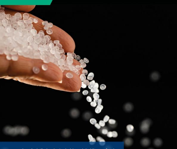
PureCycle Technologies holds a global license for the only patented solvent-driven purification recycling technology and designed to transform PP plastic waste into a continuously renewable resource. The purification process removes color, odor, and other impurities from PP waste, resulting in a virgin grade recycled plastic that can be reused multiple times.
