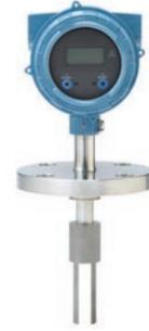
Featuring an innovative new integral transmitter, the fast-response, direct-insertion Micro Motion Fork Density Meter (FDM) offers installation flexibility with continuous, real-time density and concentration measurement in pipelines, bypass loops and tanks.
