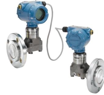
Featuring best-in-class performance and measurement stability, the Rosemount 3051S Electronic Remote Sensor (ERS™) System is engineered with flexible, digital architecture. The ERS System calculates differential pressure electronically using two pressure sensors linked together with an electrical cable. Easy to install, this safety-certified system is engineered for faster response time than traditional systems, providing you with exceptional performance in the brew kettle.
