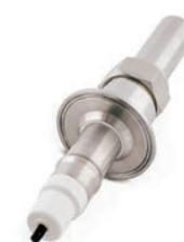
The Rosemount TF396 sensor features an ion-selective field effect transistor (ISFET) pH electrode that provides a stable pH measurement. Its rate of response can be ten times faster than glass electrodes, enabling better process control. Aging effects caused by temperature fluctuations or large changes of process pH are greatly reduced, providing longer intervals between calibration and maintenance of the sensor.
