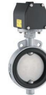
A resilient and proven valve for general purpose applications in brewing operations. The body locating holes ease installation and centering between the flanges, rounded polished disc edge gives full concentric sealing, lower torques, longer seat life and bubble-tight shut-off. No flange gaskets required. With no need to remove the actuator during seat replacement, the butterfly valve is suited for the brewing industry.
