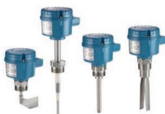
The Rosemount 2500 Solids Switch range offers the complete choice of point level measurement for bulk solids. Four different technologies are available. Rotating paddle, vibrating rod, vibrating fork, and capacitance. The switches provide flexible measurement for powders, grains, and pellets and their compact size makes them ideal for installation in all sizes of vessels and silos.
