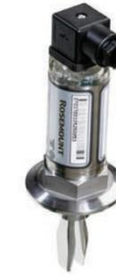
The Rosemount 2110 Level Switch offers simple and reliable level detection for compact spaces and in-pipe measurement. Hygienic certificates and all-stainless steel construction expands application capability to include sanitary processes. The vibrating fork technology has no moving parts, needs no calibration, and is virtually unaffected by process conditions.
