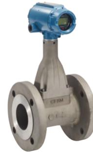
The Rosemount 8600 Utility Vortex flow meter is optimized for general purpose flow metering and utility applications including clean fluids and steam flow. The 8600 Utility Vortex meter offers enhanced reliability and simplified maintenance with superior vibration immunity without any moving parts. Installation is easy with no impulse lines or zeroing required and internal verification of both the electronics and sensor add enhanced process insight.
