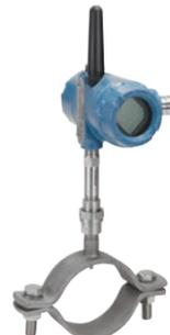
Rosemount X-well Technology provides accurate process temperature data without requiring process pipe penetration. It works by measuring the ambient and pipe surface temperatures to calculate process temperature via a thermal conductivity algorithm. X-well offers easy installation with a selection of clamp sizes and materials, providing an effective solution over a wide range of temperatures.
