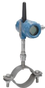
Rosemount X-well Technology provides accurate process temperature data without requiring process pipe penetration. It works by measuring the ambient and pipe surface temperatures to calculate process temperature via a thermal conductivity algorithm. X-well offers easy installation with a selection of clamp sizes and materials, providing an effective solution over a wide range of temperatures.
