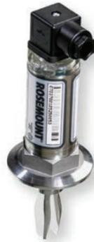
A level switch with 3-A and EHEDG standards and FDA approved materials offering reliable level detection with minimum maintenance for applications in narrow spaces. It is ideal for simple fast-fit applications and basic overflow prevention. The Rosemount 2110 has no moving parts, needs no calibration, and is virtually unaffected by process conditions. The compact hygienic stainless steel housing and plug-socket connection provides for fast-fit.
