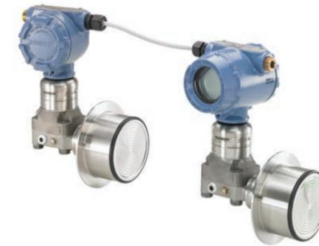
An ERS System Featuring best-in-class performance and measurement stability which calculates differential pressure electronically using two pressure sensors linked together with an electrical cable. Easy to install, this system is engineered for a faster response time compared with traditional systems to provide you with exceptional performance.
