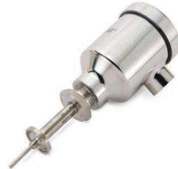
An industry-standard, resistance temperature detector (RTD). This sensor is engineered to provide flexible and reliable temperature measurements in hygienic process environments for the Dairy Industry. This RTD is designed with a Tri Clamp® sanitary endcap configuration for easy installation, and its aseptic process connection is suitable for clean-in-place (CIP), dead-pocket free, measurement applications.
