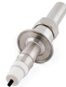
This sensor features an ion-selective field effect transistor (ISFET) pH electrode that provides a stable pH measurement. Its rate of response can be 10 times faster than glass electrodes, enabling better process control. Its short response time and increased stability provides longer intervals between calibration and sensor maintenance.
