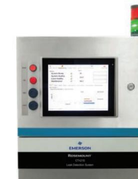
An in-line system that tests for leaks in modified atmosphere packaging (MAP) for shredded cheese applications. Unidentified leaks can impact product quality and cause waste or spoilage. The Quantum Rosemount Laser technology offers high-speed detection and automatically rejects defective packages from the assembly line. The system is easy to install and configure, minimizing disruption to the production line.
