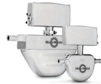
The compact, lightweight Micro Motion Filling Mass Transmitter accurately measures products with high viscosities, making it ideal for high-speed, precision measurement in yogurt filling applications. The product is 3-A and EHEDG approved.
