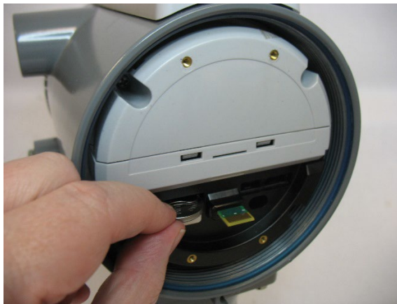
Figure 5-6. Removing/Replacing the Coin Cell Battery
