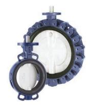
A resilient and proven valve for general purpose applications in spirit operations. The body locating holes ease installation and centering between the flanges, rounded polished disc edge gives full concentric sealing, lower torques, longer seat life and bubble-tight shut-off. No flange gaskets required. With no need to remove the actuator during seat replacement, the butterfly valve is suited for the spirit industry.
