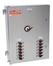
Appleton PlexPower breaks away from traditional panelboard design by transferring flame path protection from the enclosure to individual circuit breaker housings. Housings provide explosion protection for standard off-the-shelf breakers, eliminating the need for expensive special breakers, and a heavy cast and bolted enclosure allowing for simpler, faster maintenance. Lighter, compact materials, fewer long cable runs and modular design construction reduce upfront installation time and cost.
