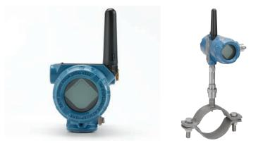
A fully wireless temperature transmitter providing stability for monitoring. When combined with Rosemount X-well<sup>™</sup> Technology and the Rosemount 0085 Pipe Clamp sensor, this transmitter can provide accurate measurement of process temperature via an in-transmitter thermal conductivity algorithm, eliminating the need for a thermowell or process penetration, significantly reducing installation time and costs.
