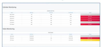
Improve OEE and Production Uptime – monitor actuator and valve performance cycles and condition preventing unexpected failures affecting availability.
