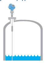
Comprehensive 2 point remote proof-testing with 94 percent coverage. Perform at the DCS, during operation, without raising the tank level to potentially hazardous levels. Minimized risk and maximized safety in minutes.
