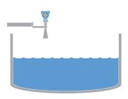
Short range measurement for sumps and flumes and long ranges including dams.
