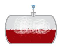
Accurate and reliable level measurement on storage or buffer tanks where there is foam, turbulence, condensation and low DC media.
