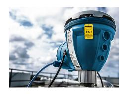
The Rosemount 5900 Radar Level Gauge is designed with functionality that lets you proof-test high alarms and verify correct product surface measurement. The Rosemount 5900 gauge allows you to combine continuous product level monitoring with proof-testing at regular intervals. It is based on a dedicated reference reflector that introduces a radar echo at a predefined position in the tank.
