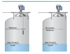
Rosemount 5900 Radar Level Gauges allow for simultaneous remote proof-testing and level measurements. Tanks that were previously difficult to proof-test during operations can now use the new innovative simulated reference reflector for this purpose.
