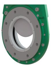
**Extend the life of your valves** with standard inlet and outlet hardened wear rings to protect the sealing elements and body from abrasive slurry. These durable Ni-Resist rings can be rotated 3 times through 4 positions to extend valve life and replacement intervals, allowing you to improve your asset utilization and process productivity.
