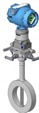
Figure 1.11: The integrated DP flow meter combines both the primary element and the transmitter into a single unit, thereby reducing potential leak points during installation and use.
