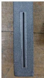
Figure 11.14: Grit-blasted surface of a Rosemount 485 Annubar primary element.
