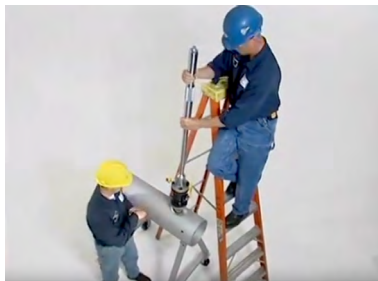
Figure 10.36: A simple hand-operated hot tapping machine.
