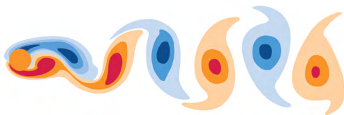
Figure 7.41: A vortex street for a cylinder in cross flow.
