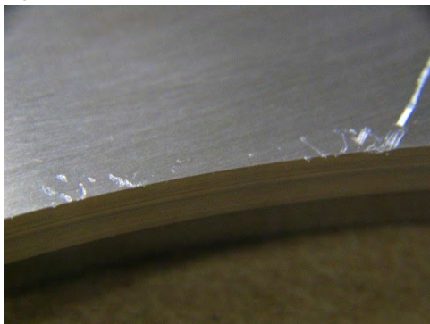
Figure 10.2: Damage on an orifice plate front surface and edge.
