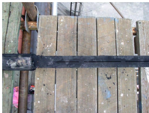
Figure 10.43: Stack primary element removed from a stack to be cleaned. Even with significant buildup of solids on the Annubar Averaging Pitot Tube, the sensing ports remained clear.
