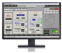
Integrated Ovation excitation capabilities provide the ability to monitor and control all plant systems from common workstations.
