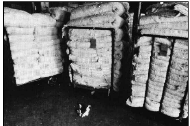
CLASS III, DIVISION 2 STORAGE AREA.
