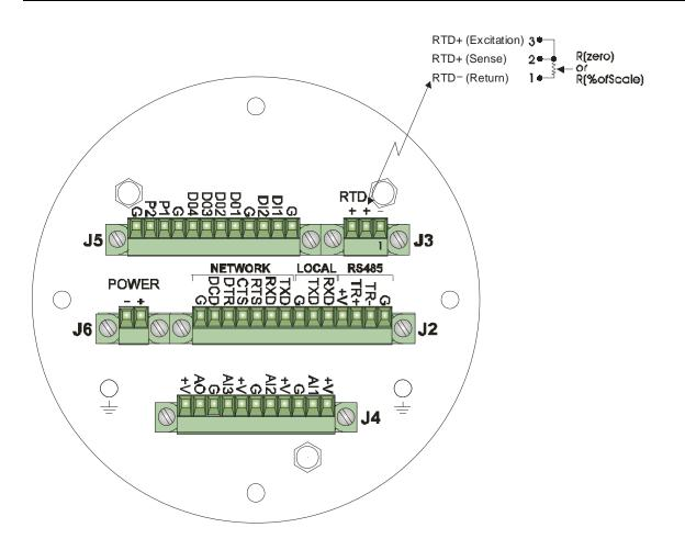
Figure 9-7. Connections for RTD Temperature Calibration – ControlWave XFC (see page 5-7 for resistor values)
