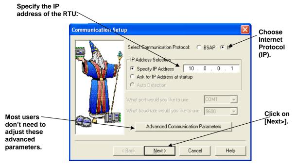
Figure 3-3. Communication Setup dialog box (IP)
