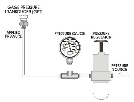
Figure 5-3. Typical Calibration Setup of GPT Using Test Pressure
