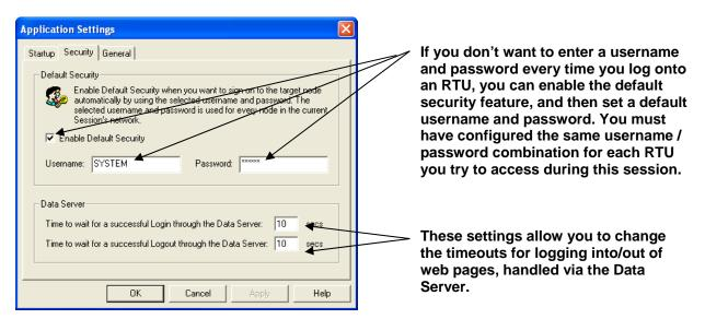
Figure 4-8. Application Settings dialog box – Security tab
