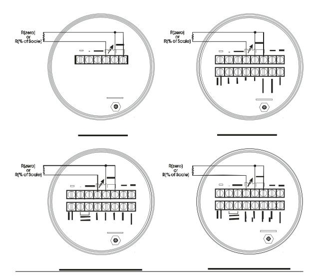
Figure 6-4. Model 3508 TeleTrans - Connections for RTD Calibration (See page 5-7 for resistor values)
