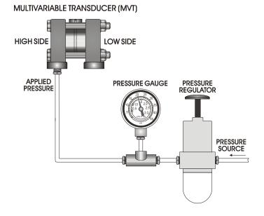
**Note**: For static pressure calibration setup, connect an identical supply pressure to the low side port of the MVT.
