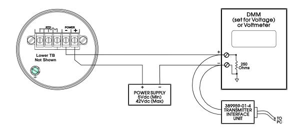
Figure 7-5. 3808 Analog Output Calibration - Voltage Measurement Diagram
