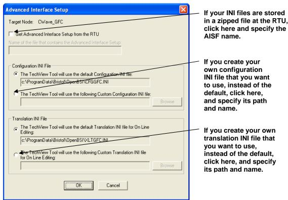
Figure A-1. Advanced Interface Setup dialog box
