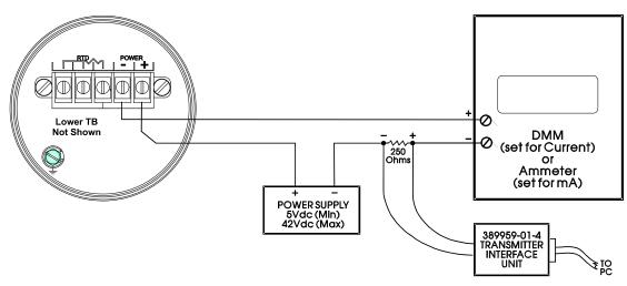
Figure 7-6. 3808 Analog Output Calibration - Current Measurement Diagram
