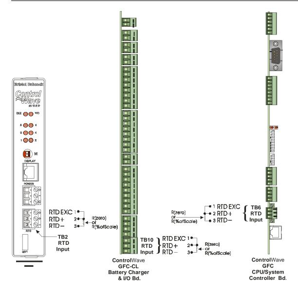
Figure 9-6. Connections for RTD Temperature Calibration – ControlWave EFM, ControlWave GFC-CL, ControlWave GFC (See page 5-7 for resistor values)
