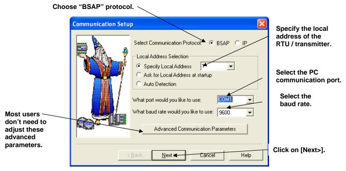
Figure 3-2. Communication Setup dialog box (BSAP)
