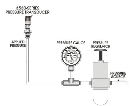
Figure 8-6. 3530-45B/-55B TeleRecorder Pressure Transducer Connections
