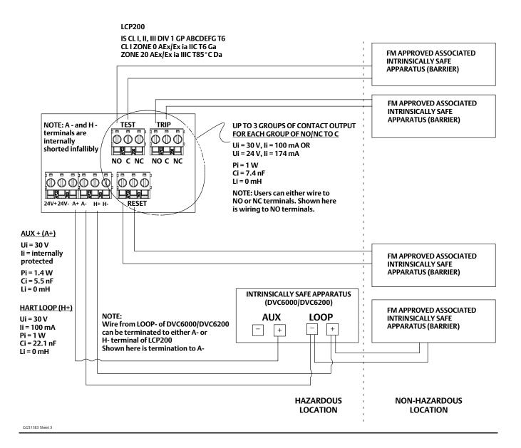
Figure 2. Intrinsically Safe, External Power 24V, FM (United States/Canada) Wiring Configuration B (External 24V Only) From Barrier to Digital Valve Controller and LCP200 See Figure 3 and Notes 1, 2, 4, 5, and 6 in Figure 4.
