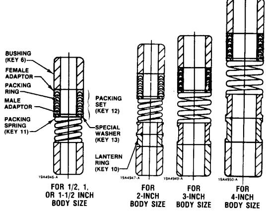
FOR 316 STAINLESS STEEL METAL **PACKING BOX PARTS** SINGLE PTFE V-RING PACKING ARRANGEMENT
