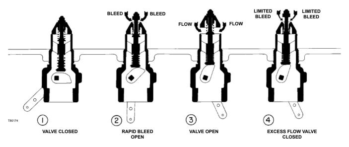
Figure 3. Operational Schematic
