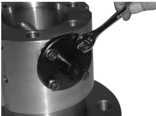
Figure 7. Bolt Up the Packing Flange
