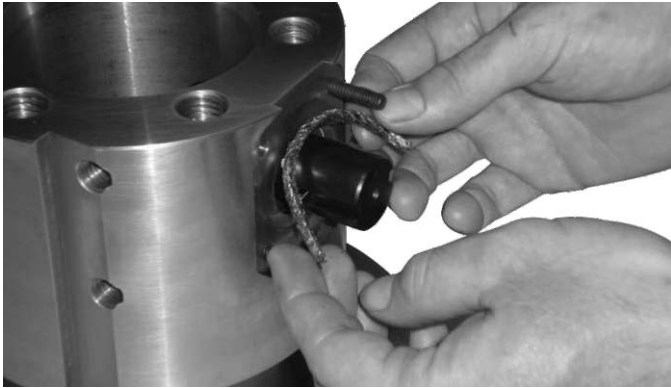
Figure 6. Use Packing Flange
