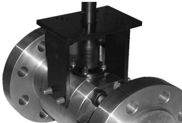
Figure 9. Position the Mounting Bracket
