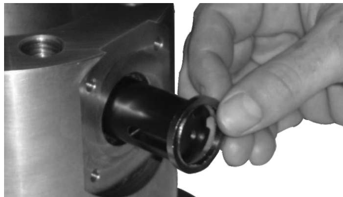
Figure 5. Insert Top End Ring
