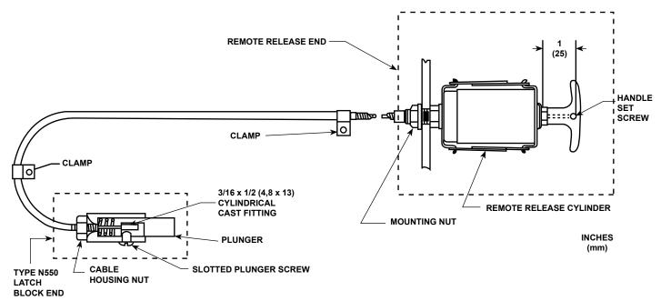
Figure 3. Type P164B Cable Release Installation Schematic
