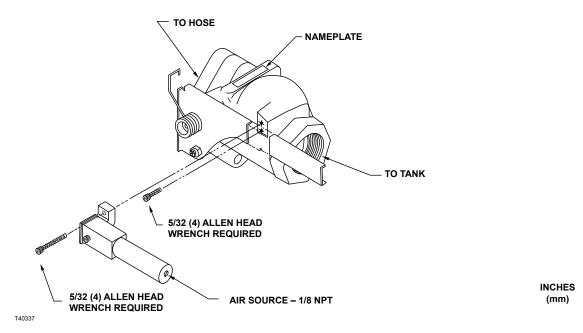
Figure 4. Type P327D Pneumatic Cylinder Installation
