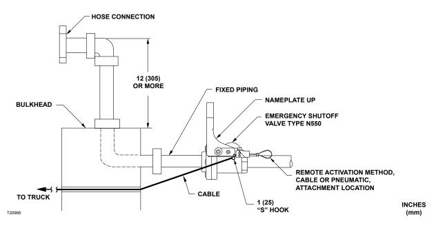
Figure 5. Motion Release Cable Installation (Optional)
