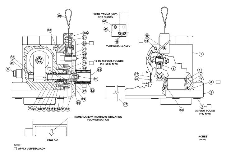
Figure 6. Type N550 Shutoff Valve Assemblies
