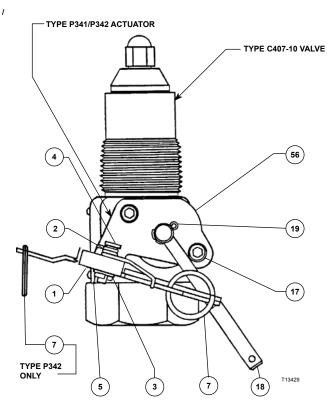
Figure 4. Type P341 or P342 Installed in Type C407-10 Internal Valve
