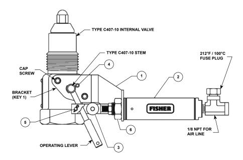
Figure 5. Type P389 Installation
