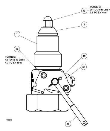
Figure 3. Type C407-10 Internal Valve Assembly
